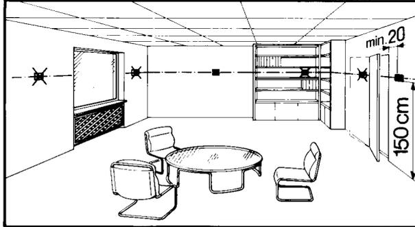
The thermostat can be fitted to most commercially available recessed conduit boxes or directly on the wall.
